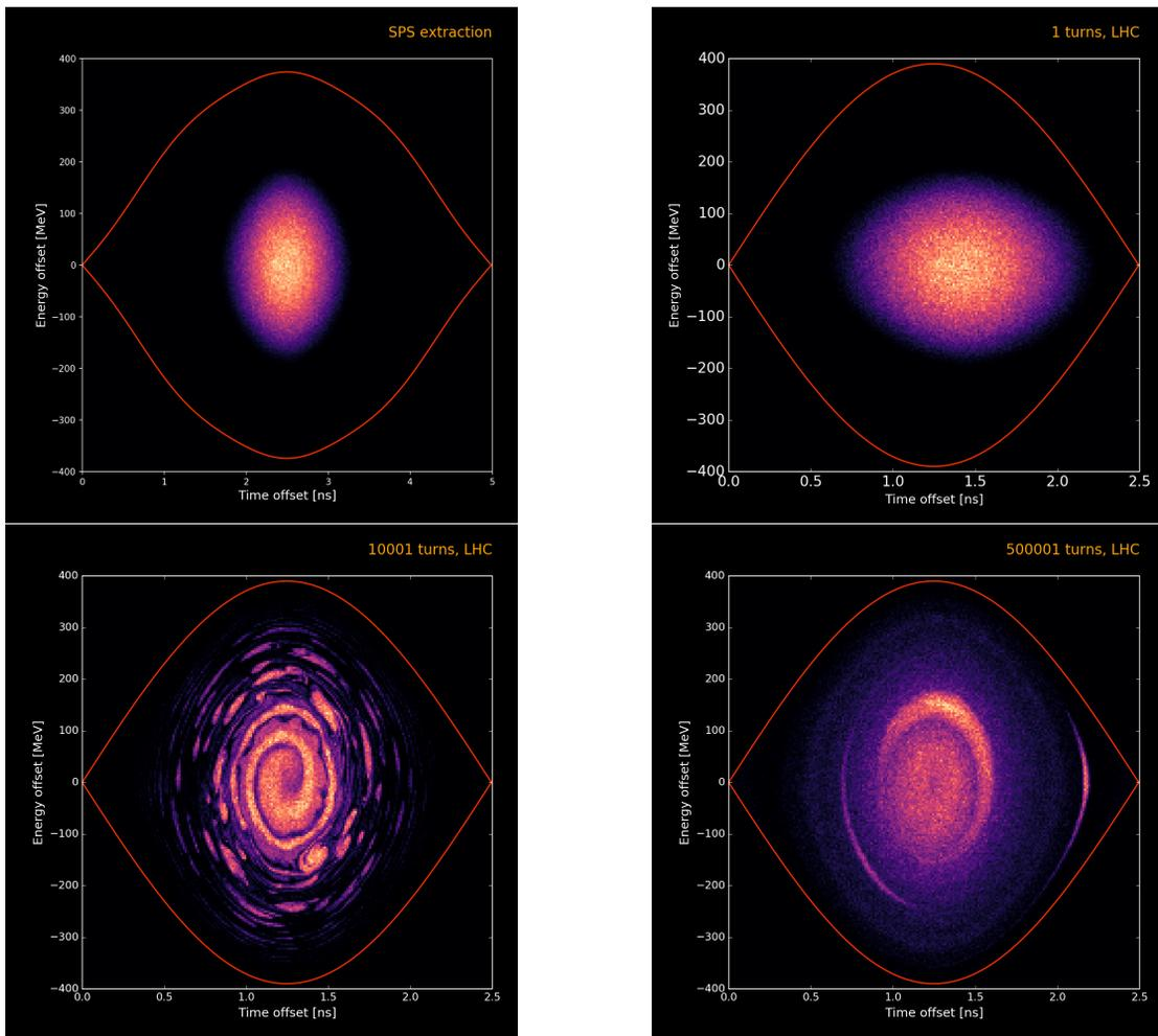
Figure 4: Formation of instability after injection at an intensity of  $1.2 \times 10^{11}$  ppb. The bunch is matched in the SPS double RF bucket (top left). At injection to the LHC with a  $25^\circ$  phase error (top right), the bunch length is 1.4 ns and the RF voltage is 6 MV. First islands form already during the filamentation process (bottom left), resulting in a more pronounced island (bottom right) eventually. A binomial distribution with exponent 1.5 was used.
